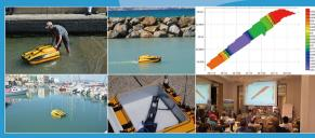
• By using unmanned boat for automatic water sampling and monitoring, a demonstration work was made in Heraklion, Greece. Integated with YSI EXO2 multi parameters sonde for online water quality monitoring. Samples were automatically took and stored in sampling box.
