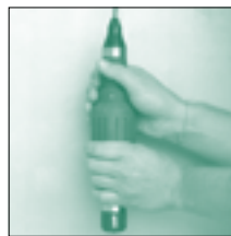
2: The switch ring is set to the pH value of the buffer (4, 7, or 10).
