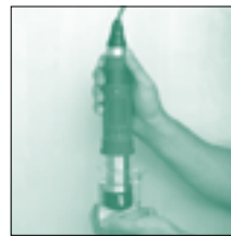
3: Zero and span is set automatically when immersed into the buffer. (Dip).
