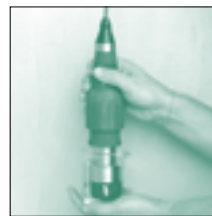
3: Zero and span is set automatically when immersed into the buffer solution.
