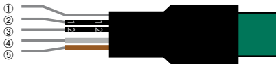
pHix ® Compact with 2 x 4-20 mA outputs, 1 for pH or redox measurement and 1 for temperature measurement.
