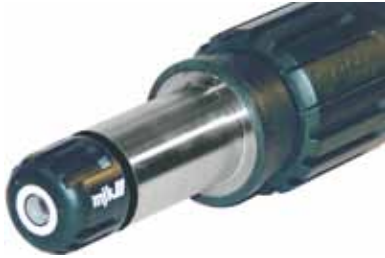
pH electrode, item no. 160310, 1 - 14 pH, 50 - 180 °F, 0 = 4.6 pH.
